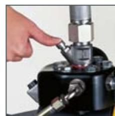
The inlet valve pushbutton ensures a high level of **operational safety**. Press it once with your thumb, and the valve is free.
